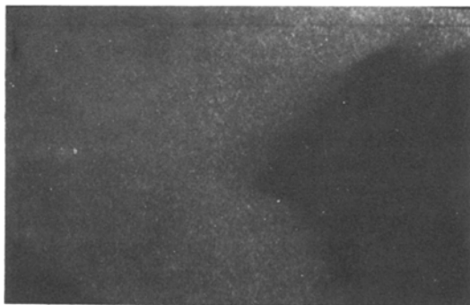
Figure 17 Dark-field image after 3 h heat treatment of the NLP 101 fibre at 1200° C in an argon atmosphere. The structure remains amorphous.
